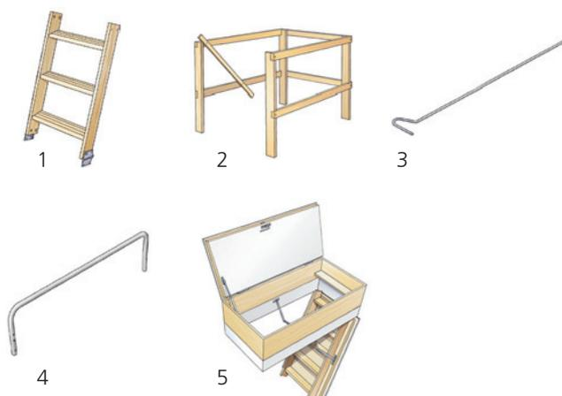
5. Upper hatch LEX D70. Noise insulating and heat saving upper hatch specially designed for today's high energy requirements. Insulation: 70mm cellular plastic. Provides, where combined with loft ladder LEX 70, a U-value of 0.20 W/m<sup>2</sup>°C. Dimensioned in accordance with the frame's outer measurements.
